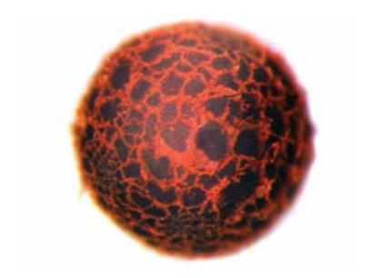
Calcium and magnesium ions are displaced from the cation exchange resin matrix with sodium ions.
